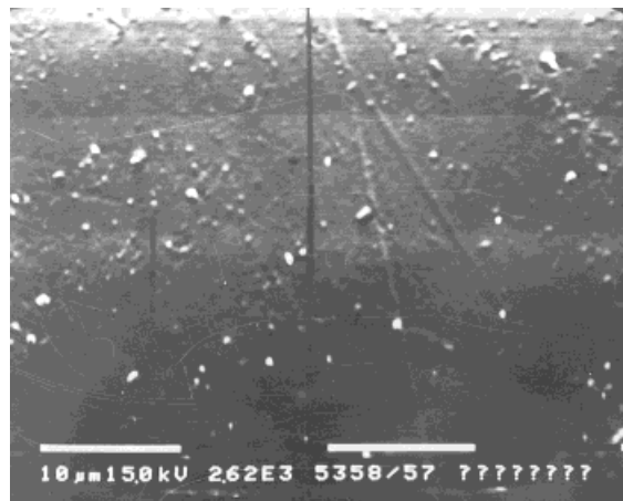
Figure 6 SEM micrograph of CTA film treated in ammonia plasma for 5 min.
